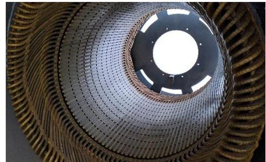
resistance and local hot spots where the insulation becomes compromised. Partial discharge then further degrades the insulation, to the point where a catastrophic event occurs, taking the equipment offline for weeks or months and posing a serious safety risk to personnel. Periodic thermal imaging scans rarely catch these failure sites in time, which is why continuous thermal monitoring is recommended.
