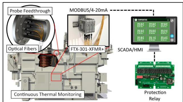
alarms for identifying temperature concerns and alerting appropriate personnel. Alternatively, the temperature transmitters can be embedded into an RTU, PLC or other control or monitoring system.
